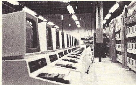
On the right of the PETs being checked out is rack upon rack of PETs being burned in. They burn 'em in for 48 hours before packing them up for shipment. Normally they have those plastic covers over the burn-in racks to make sure that the PETs are hot, thus aggravating any troubles that might otherwise turn up later.
